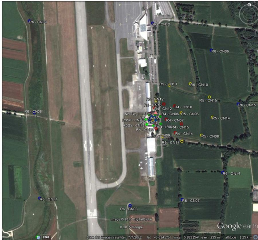
Figure A11.2: Location map of seismic data measurements (GOOGLE EARTH). Circles indicate location of seismic stations and triangles indicate MASW profile ends
