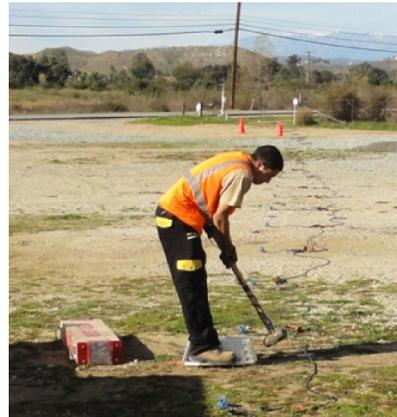
Hammer-Impact Aluminum Shear Wave Seismic Source
