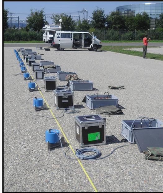
**Figure 3.1:** Example of linear array of seismological stations during a mixed active/passive acquisition survey. Each station is an independent high-resolution recording unit.
