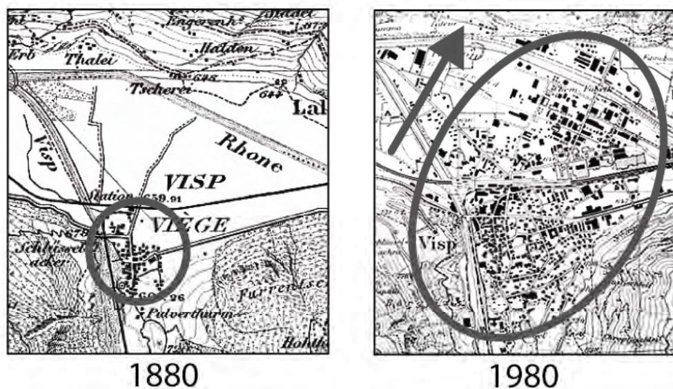
**Figure 2** Development of the village of Visp over the last two centuries. The village developed into the river plain of the Rhone, where thick layers of water-saturated sands can be found. This layer liquefied during past earthquakes in the Valais
