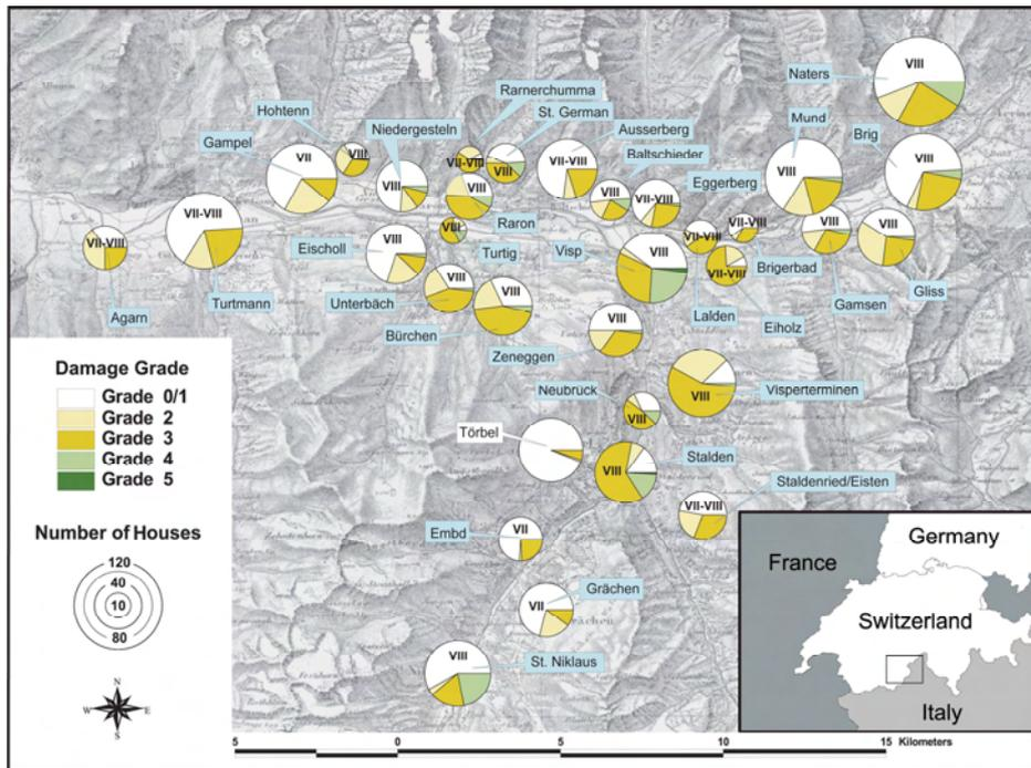
Figure 3 Damage observed during the 1855 earthquake (Fritsche et al., 2006).
