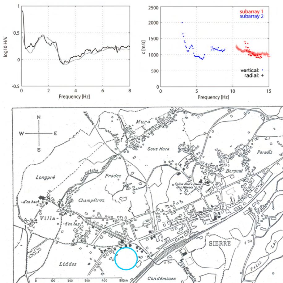
**Figure 6** H/V spectral ratios and measured Rayleigh wave phase velocity curves at the site in Sierre with increased damage during the 1946 earthquake. The map shows the city of Sierre (Wanner and Grütter, 1950). The damaged buildings are filled with black colour. The site of the measurement is indicated by the blue circle.
