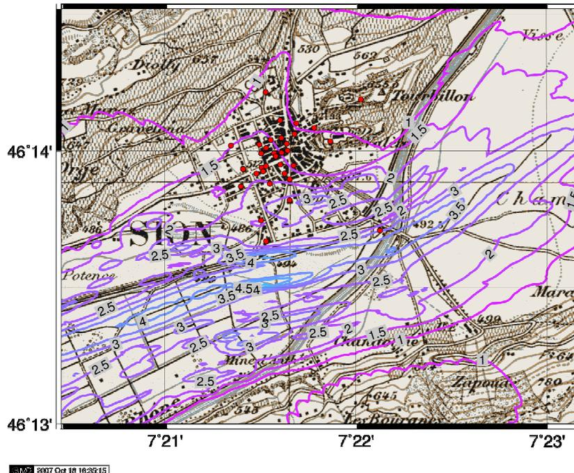
**Figure 5** Peak ground velocities obtained from the simulation of the 1946 Mw 6.1 earthquake normalized to a reference site (modified from Roten et al., 2008). Red dots show the location of buildings that suffered damage during the event (from Fritsche and Fäh, 2008). The map dates back to 1933.
