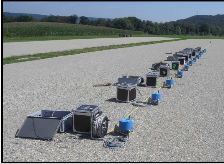
Fig. 1. Example of linear array of seismological stations during a mixed active/passive acquisition survey. Each station is an independent high-resolution recording unit.
