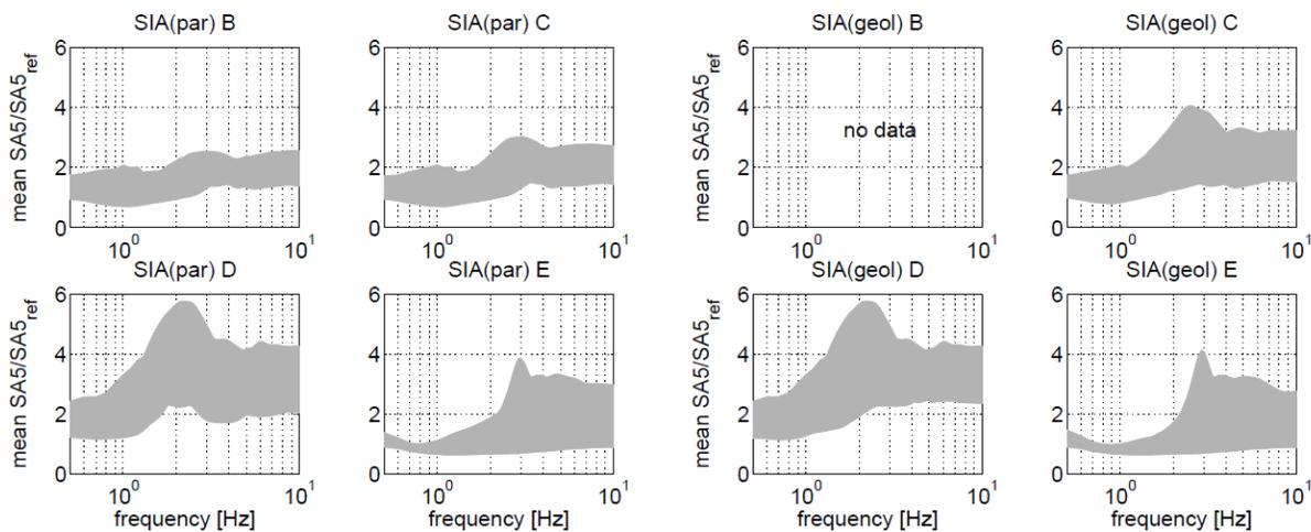
**Figure 2.** Range of mean spectral amplification (5% damping) from 1D numerical modeling, for site classes defined using parametric (left) and geologic/geotechnical (right) definitions of site classes (Steimen, 2004).
