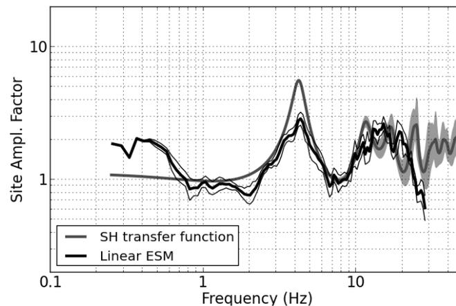
**Figure 6**, Example of empirical Fourier amplification functions (ESM, in black) and numerical modeling results (in gray) from the SED station and site characterization databases. These data are the base for the calibration of the site response factors for the different ground types.
