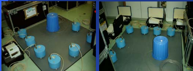
Laboratory huddle test Le3D-5s for relative calibration - D07.05
