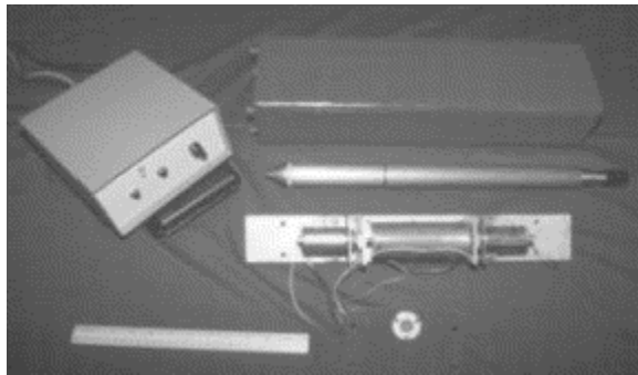
Fig 13.14: AutoSeis components, from left, control box, source frame, typical seismic cone, and internal chassis.
