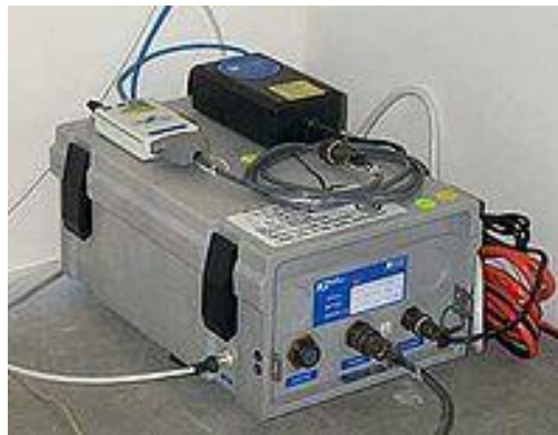
Fig 7.10: This model is a K2 made by Kinemetrics and part of the Pacific Northwest Seismograph Network.
