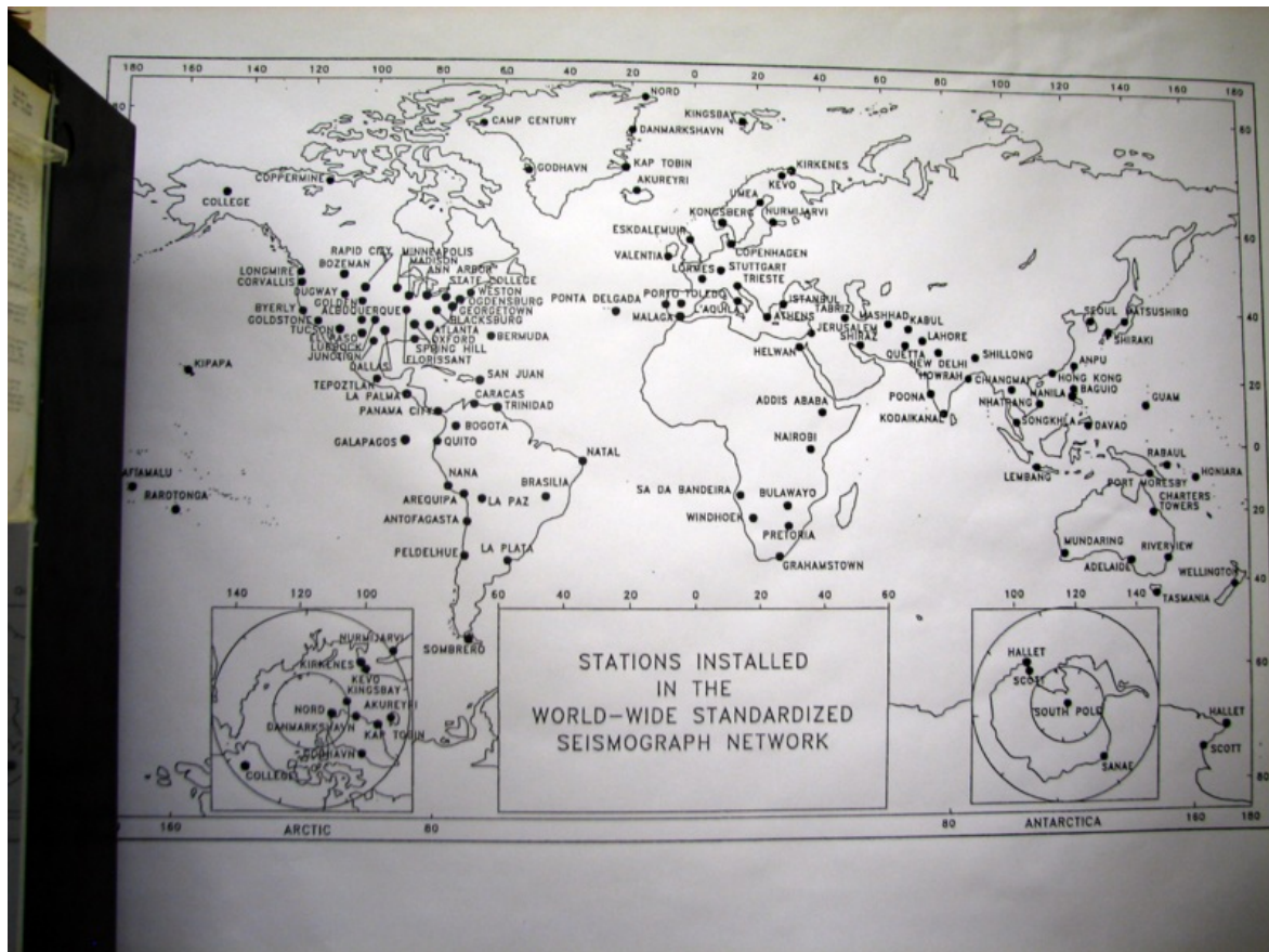
Fig. 3.10 – World-wide standardized seismograph network (WWSSN) established in the early 1960s. It used analogue short-period (1 s) and long-period (15 or 30 s) 3-component standardized seismographs and crystal clock. More recently (1980-1990s), the WWSSN has been gradually replaced by global initiatives that have utilized broad-band digital instruments.
