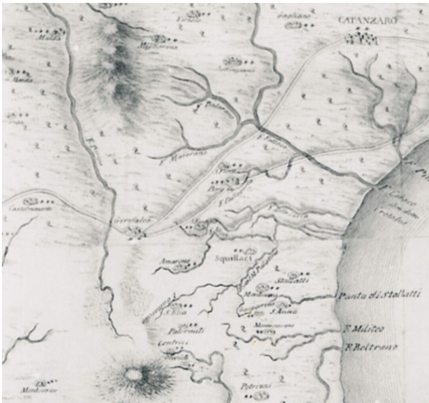
Fig. 2.1 - Detail of Schiantarelli's map of the the 1783 Calabrian earthquake: different symbols are used for villages according to the amount of damage (from Musson, 2006).
