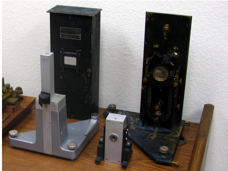
Fig. 3.14 - The short-period Wood-Anderson torsion seismometer, showing cover and sensitivity mirror in place (left) and the same without cover, showing damping magnet, lens etc. (right).
